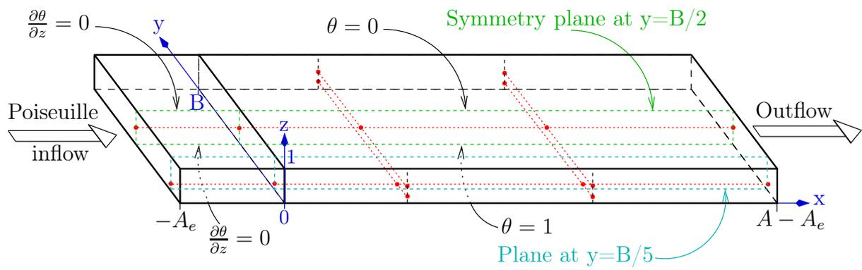
Figure 1: Geometry and thermal boundary conditions on the top and bottom walls (the vertical lateral walls are adiabatic). The red dotted lines are the lines along which  $\theta$ ,  $u$ ,  $v$  and  $w$  profiles and their extrema are calculated.
